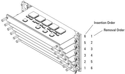
**5** Seat the modules then rotate the ejector tabs to the locked position. Repeat for all modules or filler panels.
