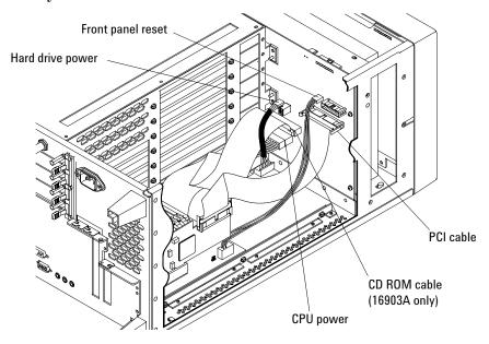
**4** Remove screws from the back of the CPU tray using a Torx T-10 screwdriver.
