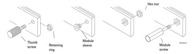
The 16900A/16902A logic analysis system comes with a set of 6 replacement thumb screws (16900-68713), and the 16903A logic analysis system comes with a set of 2 replacement thumb screws (16903-68713).
