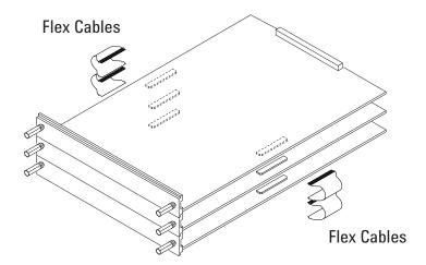
**1** Insert the lowest card about 1/3 of the way into the desired logic analyzer frame slot.
