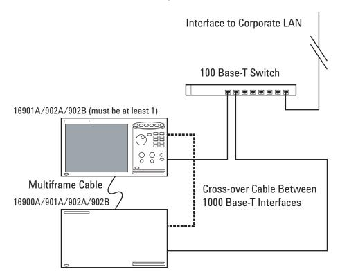
When you have only two frames in the simple 100 Base-T multiframe configuration (see page 87), you can gain performance by connecting a crossover cable between the frames' 1000 Base-T ports and configuring these ports with static IP addresses.
