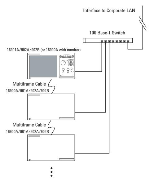
In the simple 100 Base-T multiframe configuration, all of the frames are connected to the network using their 100 Base-T LAN port.
