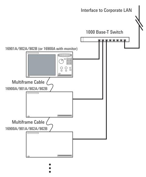
In the simple 1000 Base-T multiframe configuration, all of the frames are connected to the network using their 1000 Base-T LAN port.
