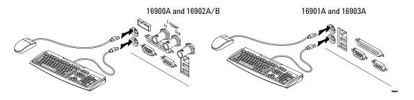
**2** Connect a monitor to the back of the 16900A. A second monitor on the 16901A, 16902A, 16902B, or 16903A is optional.
